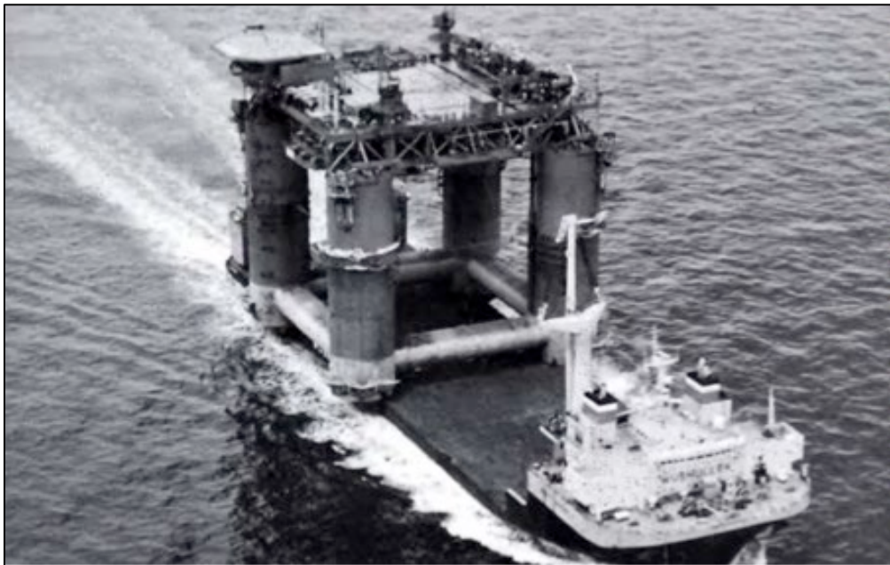
Figure 1.19. Aboard Mighty Servant III in the spring of 1989, the hull and topsides of the completed Jolliet TLWP are dry-towed from the platform's fabrication site in Singapore to a shipyard in Pascagoula, Mississippi, then on to the Green Canyon
