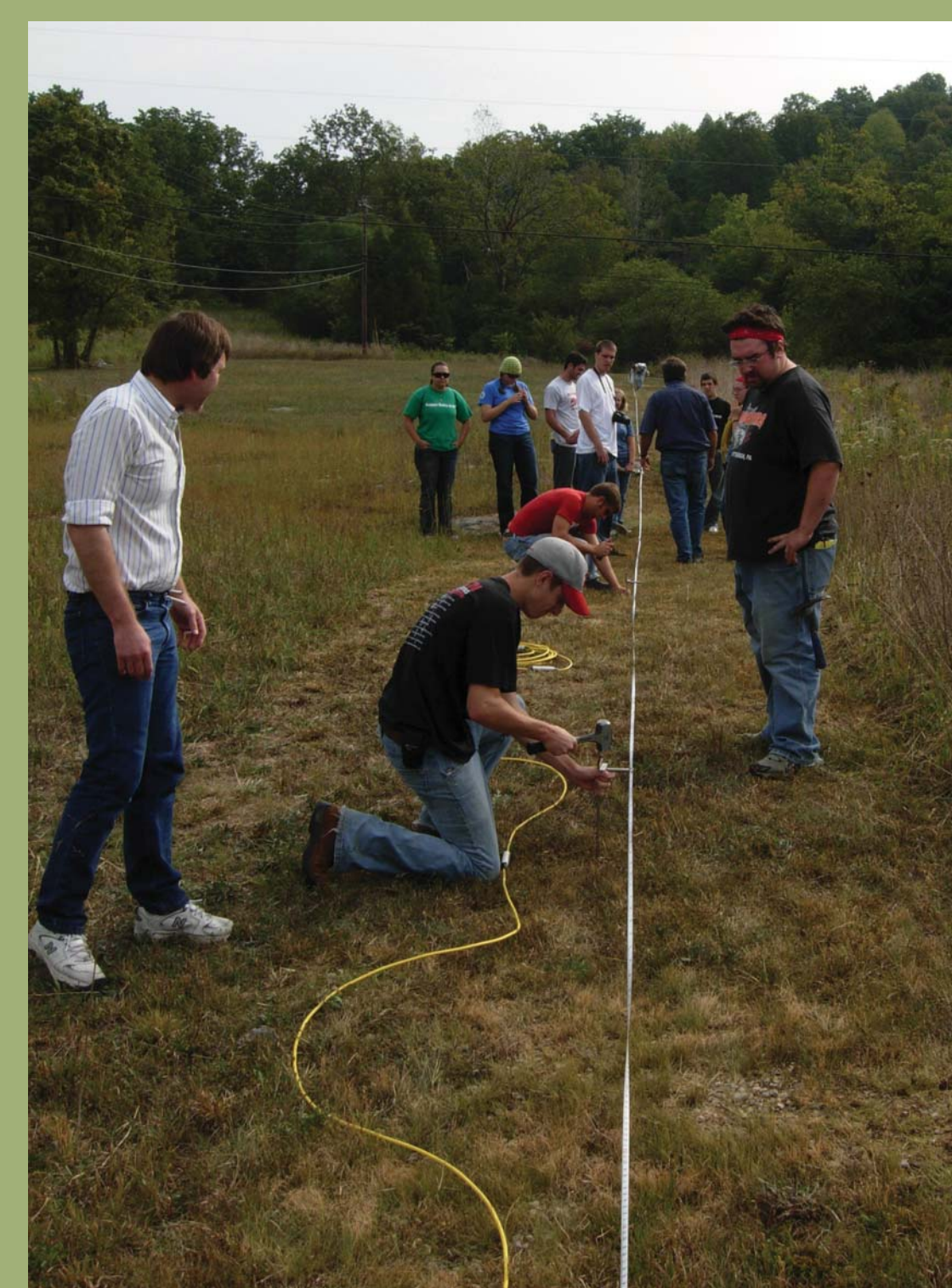
Whittenberg University students looking for cave passages using electrical resistivity testing.
