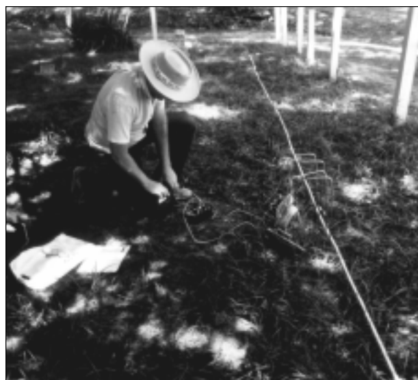
Figure 6. An electrical resistivity survey using a Gossen resistivity meter. Scott Air Force Base. (NPS, n.d.)
