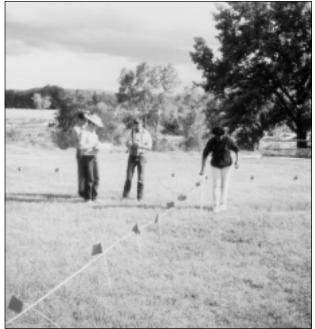
Figure 4. A magnetic survey using a GEM 19 magnetometer. Fort Laramie National Historic Site. (NPS, 1993)
