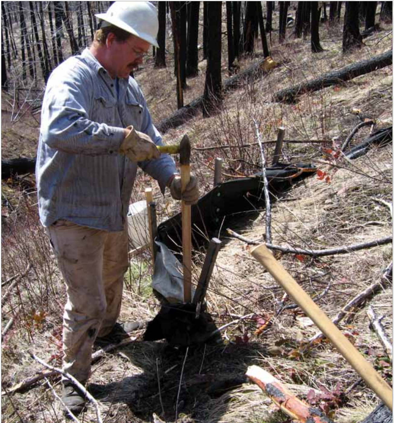
Bob Brown, hydrologist with the U.S. Department of Agriculture Forest Service, repairs a silt fence after the 2003 Myrtle Creek Fire on the Idaho Panhandle National Forest. The silt fences in this area were used to measure the effectiveness of straw mulch, hydromulch, and natural needle cast on reducing erosion after the fire.
