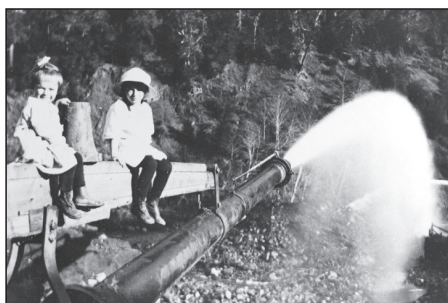
Crowin children next to hydraulic giant drive at a placer mine at Mule Creek, early 1900s
