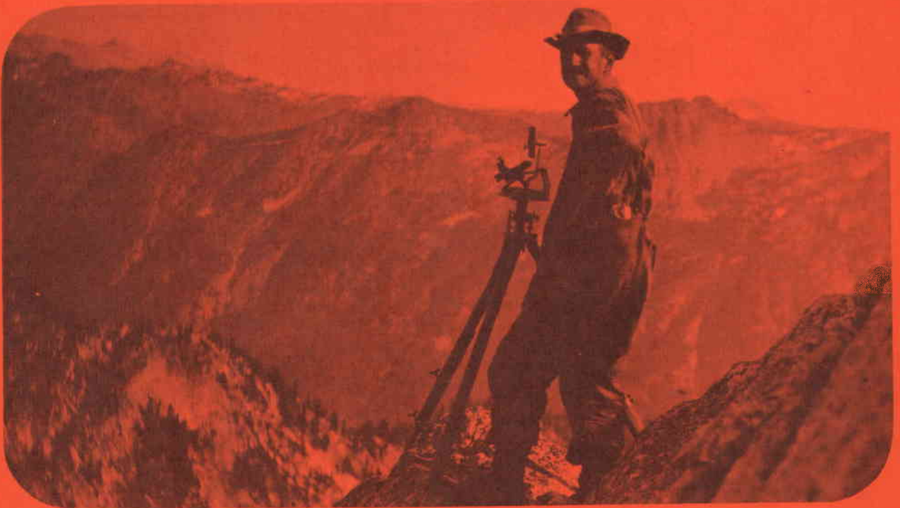
In 1914, surveyors called this "typical mountain work in the West." The mountains are in Washington State. The instrument, a solar compass with telescopic attachment, is being used by Jerry Campbell.
