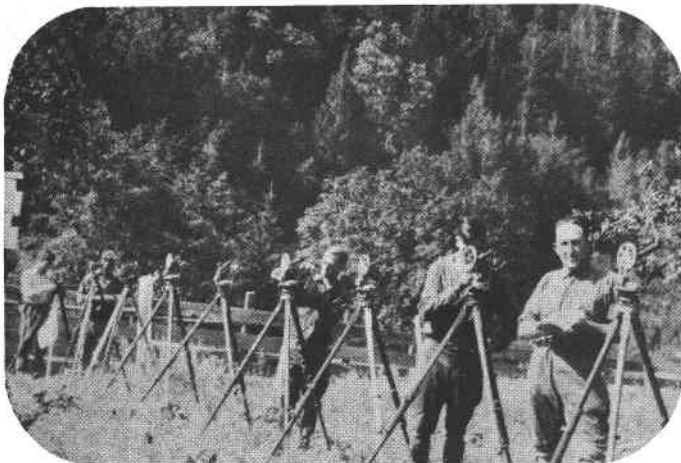
On a weekend morning, surveyors often adjusted the solar attachments on the meridian. The date of this photo is 1925.
