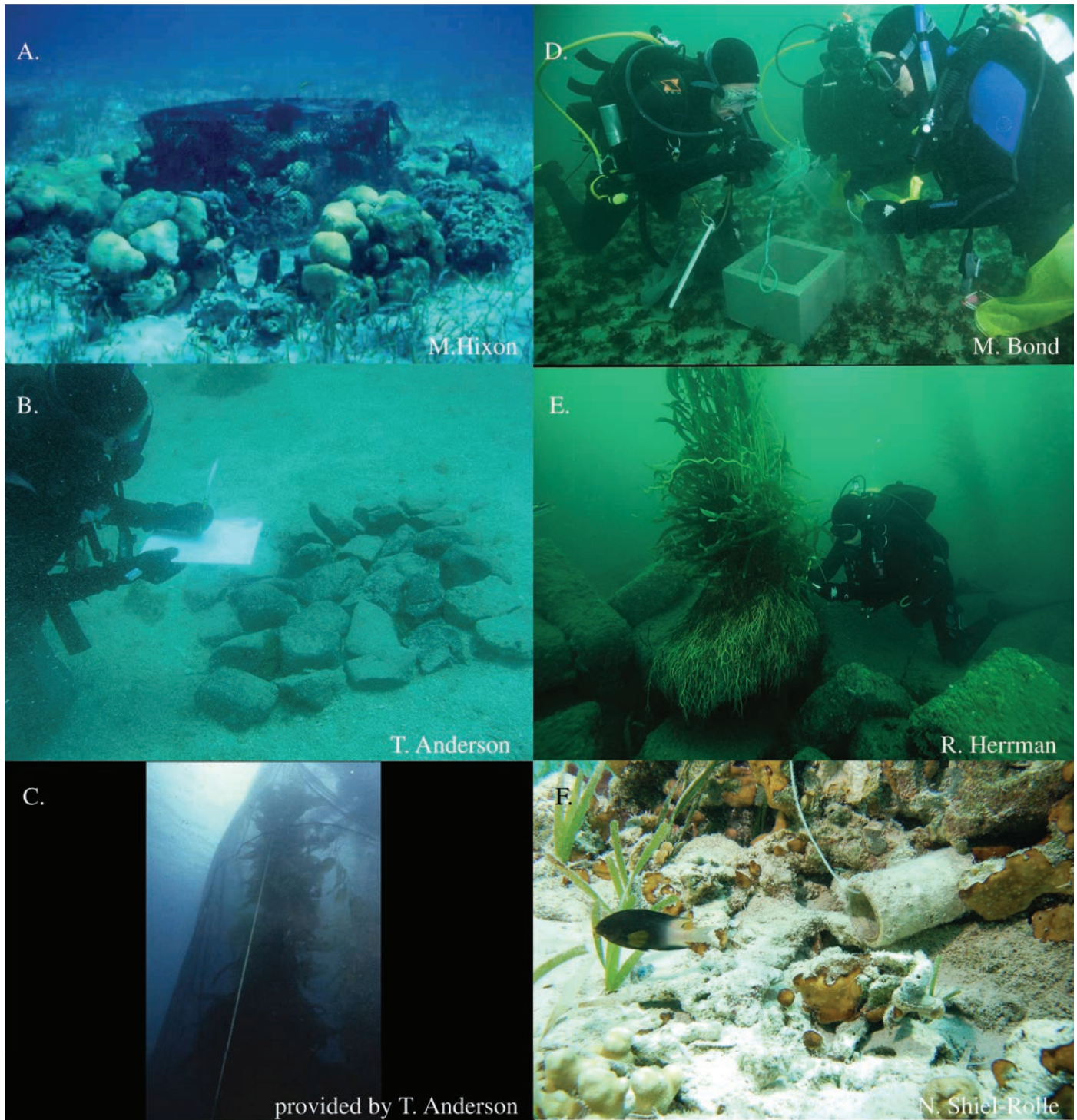
FIGURE 1. Habitat manipulations to create independent isolated experimental treatment levels (e.g., density levels, refuge availability) from natural substrata: (A) corals, (B) rock, (C) kelps; and artificial substrata: (D) cinder blocks, (E) concrete rubble, (F) tubes. (Photo credits given in each image.)
