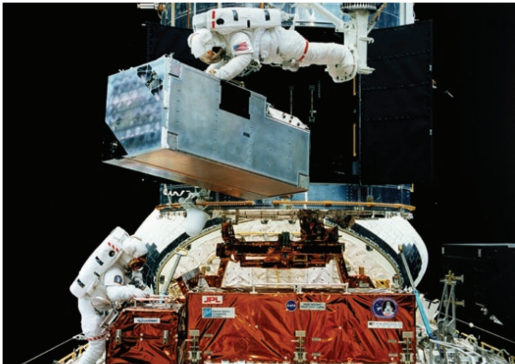
Figure 1.3-4. Astronaut Kathryn C. Thornton (top)—anchored to a foot restraint on the end of the Remote Manipulator System (RMS) arm in Endeavour’s open bay—maneuvers the Corrective Optics Space Telescope Axial Replacement (COSTAR) into position for installation in December 1993. Thomas D. Akers is at lower left. (NASA image STS061-47-014, http://images.jsc.nasa.gov/lores/STS061-47-014.jpg .)
