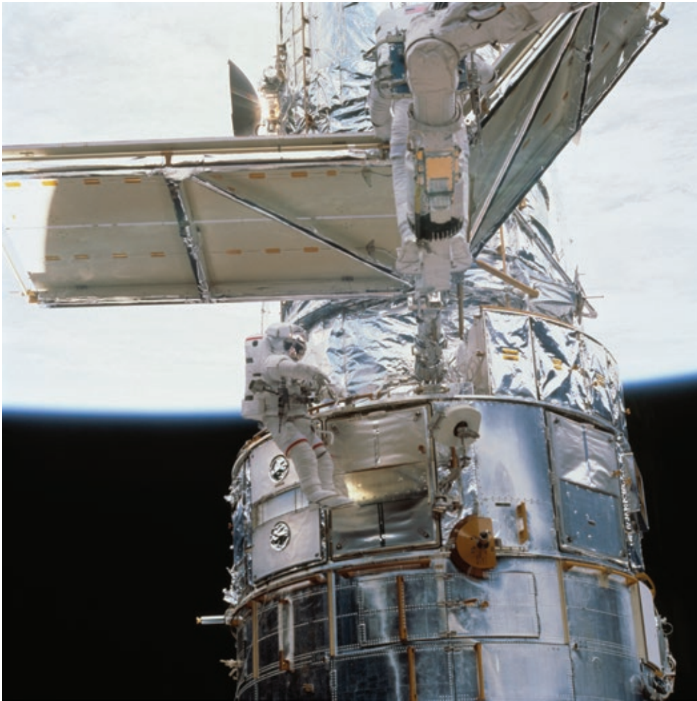
Figure 2.6-1. Astronaut John M. Grunsfeld, payload commander, is anchored by a handrail on the Systems Support Module while replacing one of Hubble's two second-generation solar arrays in 2002. Above Grunsfeld is astronaut Richard M. Linnehan, mission specialist, whose legs are visible on a foot restraint at the end of the Space Shuttle Columbia 's Remote Manipulator System (RMS). They are installing a new, third-generation solar array known as SA3. (NASA image STS109-715-038, http://spaceflight.nasa.gov/gallery/images/shuttle/sts-109/html/sts109-715-038.html .)
