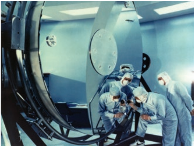
Figure 1.3-3. The 94-inch (2.4-meter) primary mirror for the Space Telescope on a transport frame in 1982, just after it was vacuum electro-coated with its reflective aluminum surface and then over-coated with a transparent layer of magnesium fluoride. (NASA image MSFC-75-SA-4105-2C, http://mix.msfc.nasa.gov/abstracts.php?p=1619 .)
