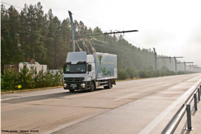
Figure 9-2: Proposed Catenary System for I-710 Zero-Emissions Corridor (Source: Siemens Mobility).
