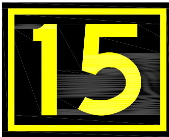
b. Runway Location Sign
