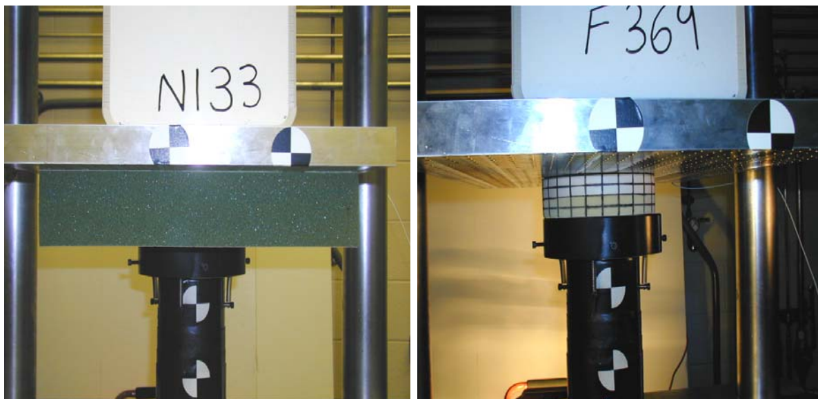
FIGURE 2-4. TYPICAL CUSHION TEST SETUPS
