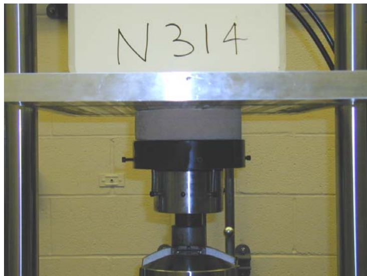
FIGURE 2-10. TYPICAL CUSHION STATIC TEST SETUP
