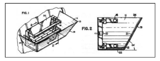
"The housing encloses the light source or sources but provides a substantial upwardly facing opening for the walking or flying entry of flying insect pests." ('690 Patent, col. 2, II 62-65; and col. 2, II. 9-15 & 24-25, col. 8, II. 40-43). "Correct placement increases insect capture through direct radiation of light and reflection of light onto either a vertical or horizontal surface (ceiling)." col. 4, II. 21-24.
