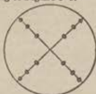
Figure 3-4. Cross section of circular stack showing location of traverse points on perpendicular diameters.
