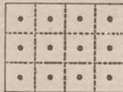
Figure 1-5. Cross section of rectangular stack divided into 12 equal areas, with traverse points at centroid of each area.
